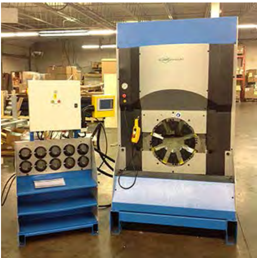
JGB Enterprise's Techmaflex PES-500 Large Bore Hose Assembly Machine allows for crimping capabilities of up to 12".
