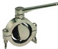
The 5102 series is a patented clamp butterfly valve. This clamp valve is an incredible 1-3/8" wide on all sizes. The valve will fit into ¾" of line space. The grooved clamp housing connects directly to clamp style fittings. Easy assembly by removing the wing nuts and using a hex key for the handle to secure and seal the housing onto your lines.
